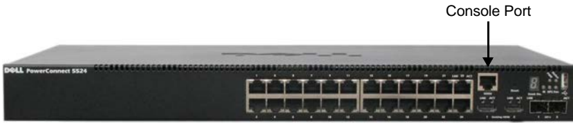
Figure 5-1. Front-Panel Console Port
